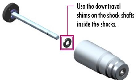
Use the downtravel shims on the shock shafts inside the shocks.
