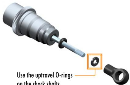
Use the uptravel O-rings on the shock shafts.
