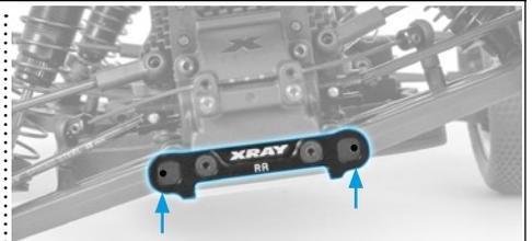
We recommend to use the suspension arm mounts in the outer position which will increase the car stability but will eliminate the drive shaft collision with the diff outdrives.
