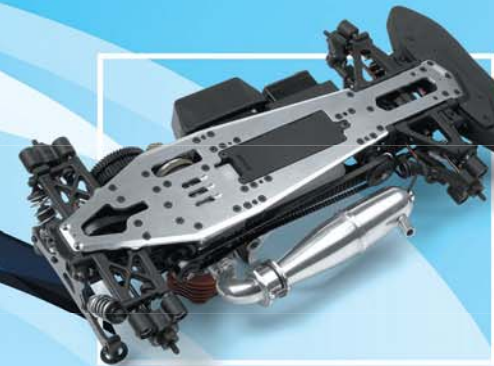
CNC-machined 3mm Swiss 7075 T6 chassis
