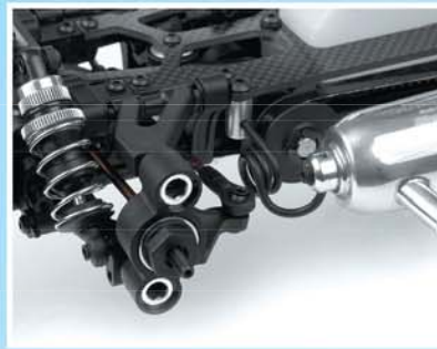
Optimized nitro touring car suspension geometry
