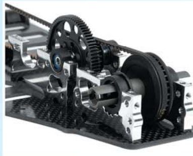
New rear split bulkheads for more rear flex
