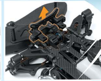
Quick & easy access to front differential
