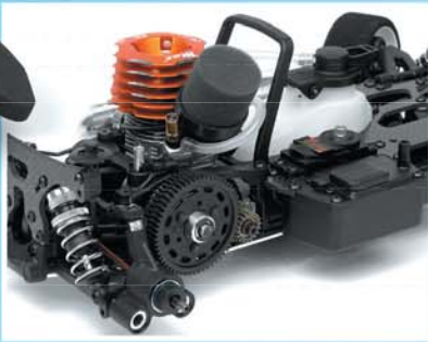
Radio box with Quick-Exchange system for crystal
