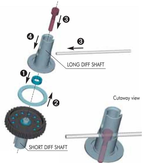
**ALWAYS HOLD THE DIFFERENTIAL VERTICAL DURING ASSEMBLY, SO THE PARTS STAY IN ALIGNMENT AND THE DIFF BALLS DO NOT FALL OUT.**
