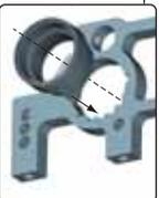
To remove holder, press out with tool as shown.
