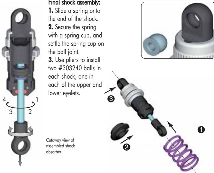
Cutaway view of assembled shock absorber
