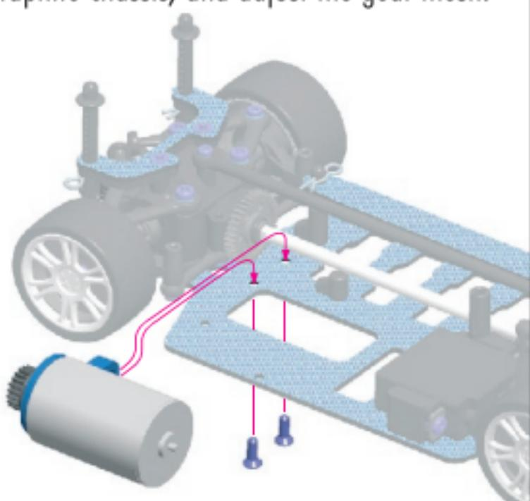
5. Gently tighten the motor mount screws.
