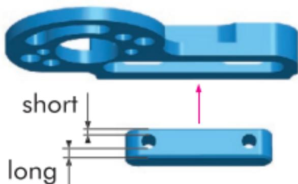
2. Attach the motor to the alu. motor holder with the screws provided with the motor.
