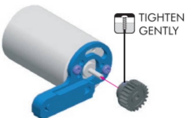
4. Attach the motor mount to the M18 graphite chassis, and adjust the gear mesh.
