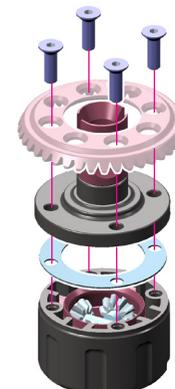
Tighten the screws equally but do NOT tighten them completely. Finish tightening in this order.
