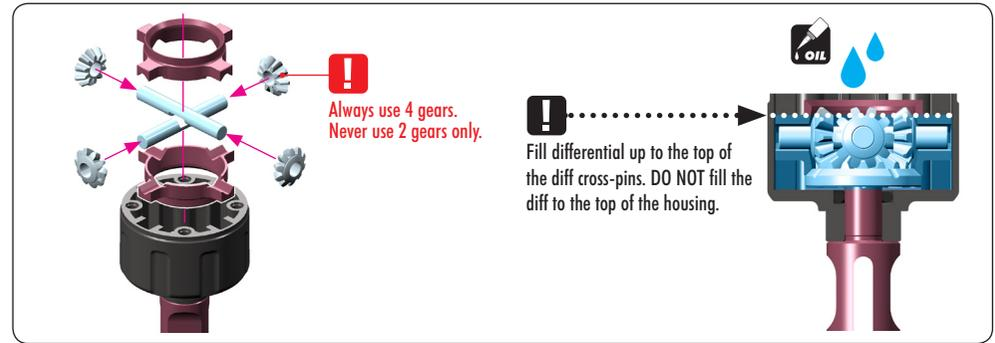
TO ENSURE YOU HAVE THE SAME AMOUNT OF OIL FROM REBUILD TO REBUILD, DO THE FOLLOWING:
