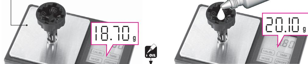
1 Put the diff (without oil) on the scale and check the weight (approximately 18.70g)
