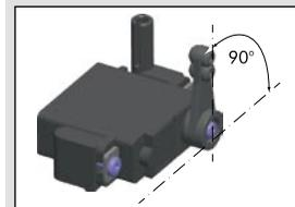
3. Attach the servo mounts to the M18 chassis.
