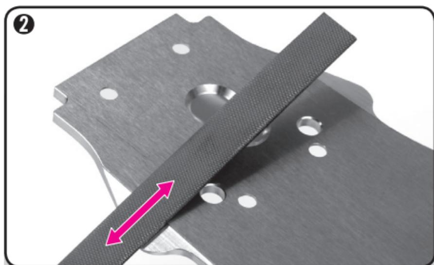
Using a file, slightly file the highlighted area under an angle on both left & right sides from the top of the chassis.
