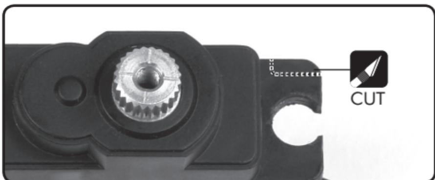
Use a sharp hobby knife and remove the edge of the servo holder as shown.
