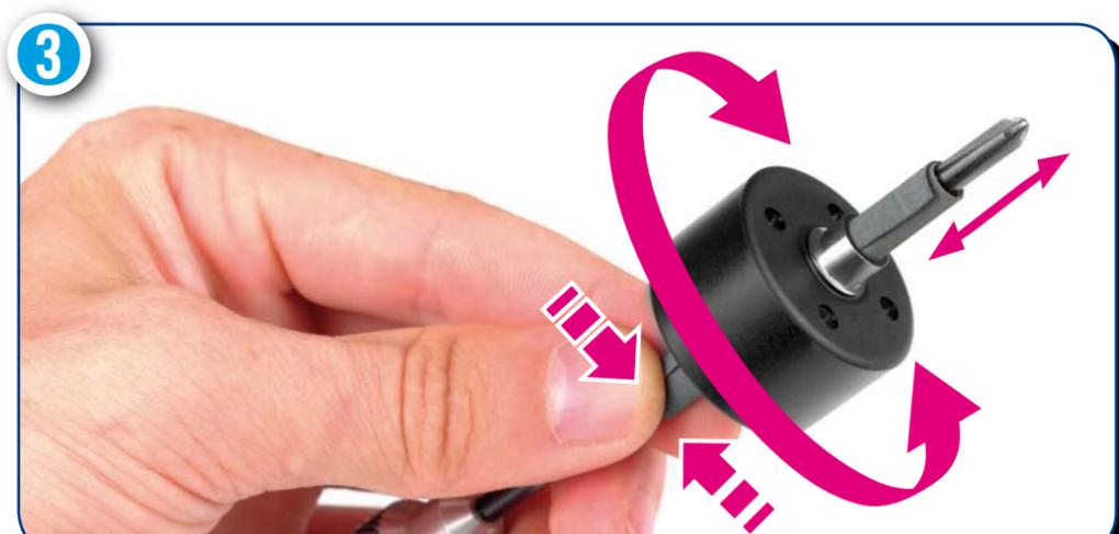
Insert the shaft or screwdriver with the rolled sandpaper into the diff case and follow the same procedure, move the shaft in and out and turn inside the diff case. Use a drop or two of light oil on the sandpaper (if desired) for smoother polishing. After finished polishing, carefully clean the parts to remove any residue or metal filings. Perform this on all the diff cases.
