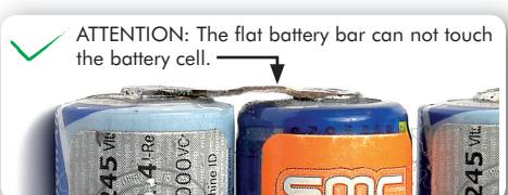
**ATTENTION:** The flat battery bar can not touch the battery cell.
