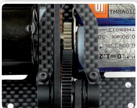
New XRAY 3.5mm narrow pinion gear with standard XRAY spur gear. There is greater distance between the pinion gear and battery bar. Note that the battery bar is flat.
