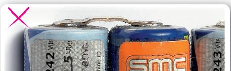
A domed battery bar may contact the pinion gear. We therefore recommend using a flat battery bar, or flatten the domed battery bar.
