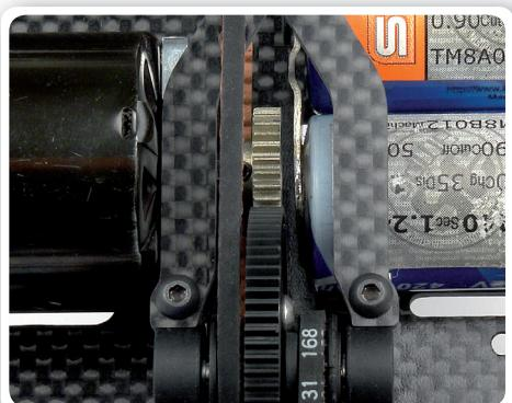
New XRAY 3.5mm narrow pinion gear with new XRAY offset spur gear. The new spur gear is more offset so it is farther away from the battery bar. Note that the battery bar is flat.
