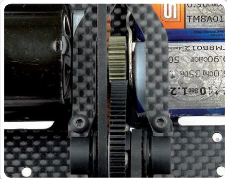
Standard 5mm wide pinion gear and standard XRAY spur gear. The pinion gear is very close to the battery bar. Note that the battery bar is flat.
