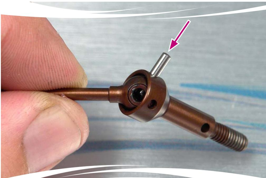
Then install pin into the drive axle in order to connect the drive axle to the shaft.
