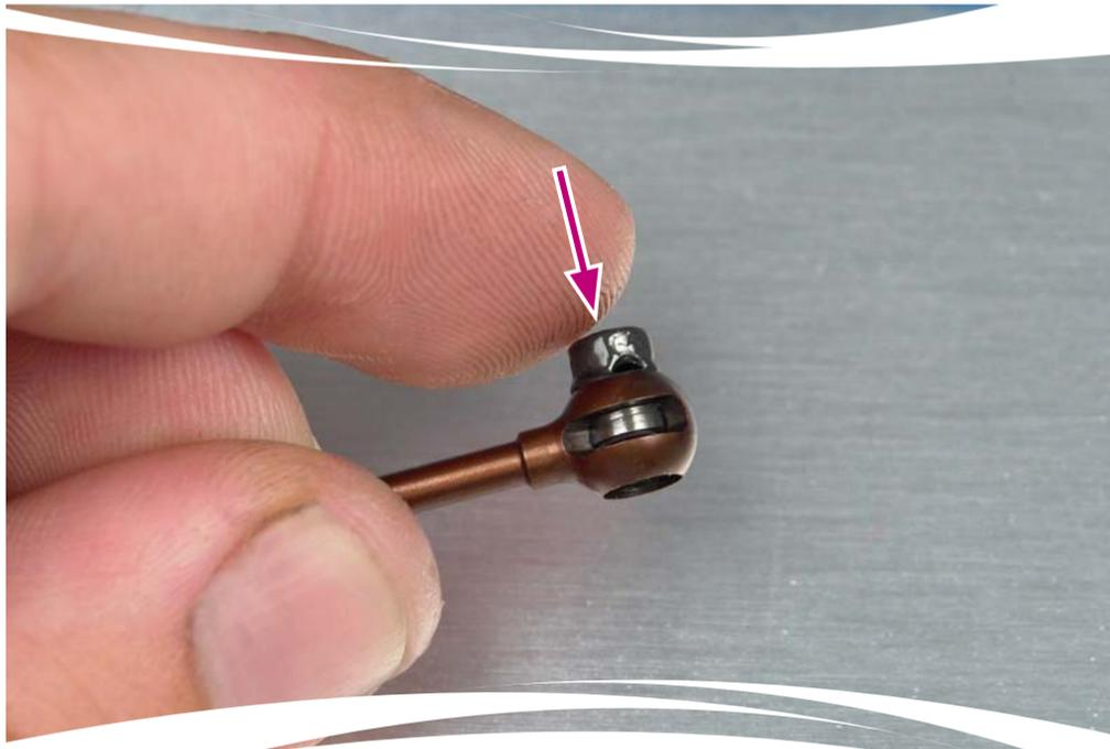
When building the drive shafts, start by greasing the coupling and inserting it into the shaft as shown.
