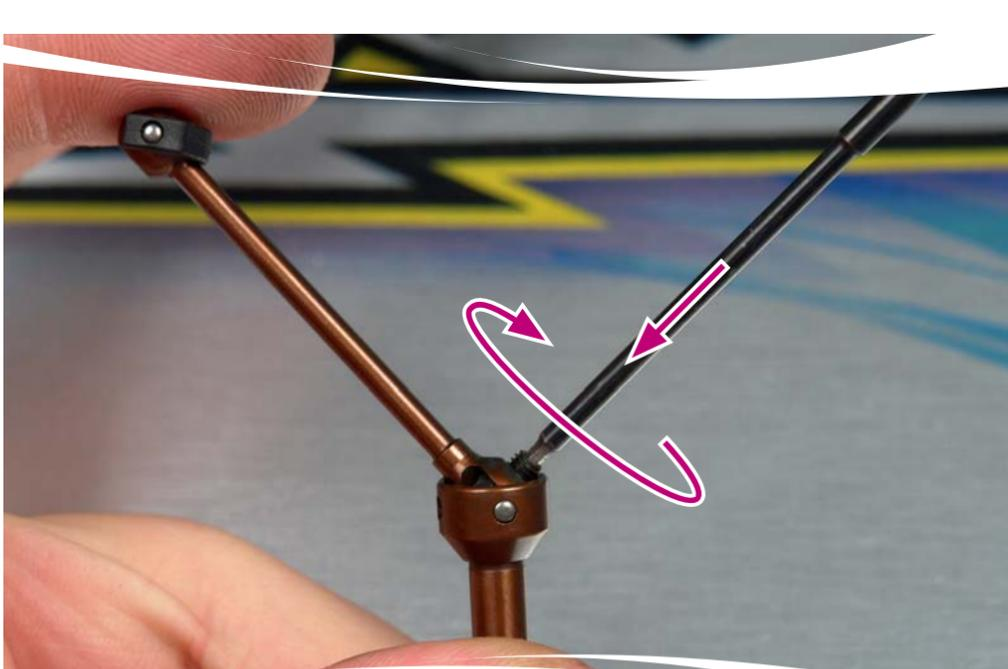
After applying threadlock to the screw, install the screw as shown. Remove any excess threadlock.
