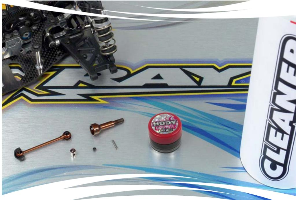
We strongly recommend using #106210 HUDY Graphite Grease for the drive shaft coupling, especially for the front drive shafts. When the coupling is not greased it may cause wheel vibration when full steering is used.
