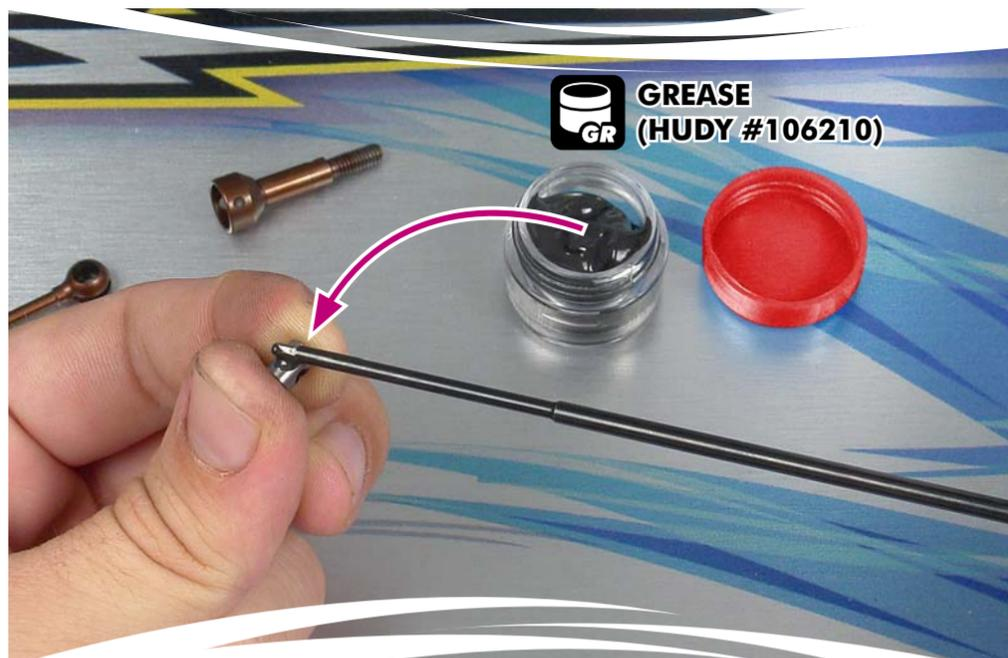
Therefore it is very important to grease the couplings very often in order to remove wheel vibrations.
