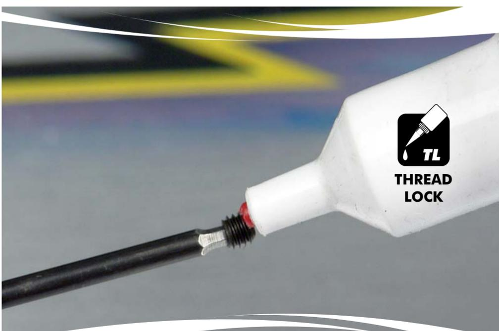
It is very important to use thread lock for the hex screw, otherwise the screw may unscrew. Use only a small amount of medium-grade (blue) thread lock on the screw.
