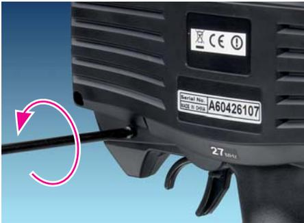
1. Using a small Philips screwdriver, remove the indicated screw from the back of the transmitter as shown. By default, the screw is in position #1 (away from the trigger).
