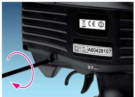
4. Using a Philips screwdriver, install the screw into position #2 (toward the trigger) as shown. Do not overtighten the screw or you will strip the plastic.
