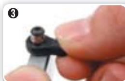
Lift ball joint until it snaps into place over pivot ball. Ball joint should move freely.
