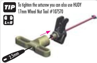
**TIP** To tighten the setscrew you can also use HUDY 17mm Wheel Nut Tool #107570
