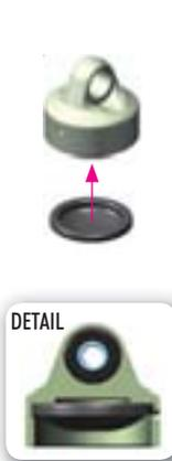
**4** Install the shock membrane into the groove in the upper shock cap.
