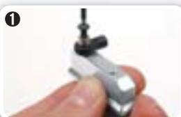
Place the pivot ball on the ball joint and use a screw to tighten it to an engine mount or some other part.
