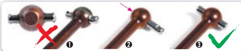
Do not use drive shafts when the pins are worn.
