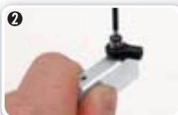
Tighten screw until pivot ball is tight against block.
