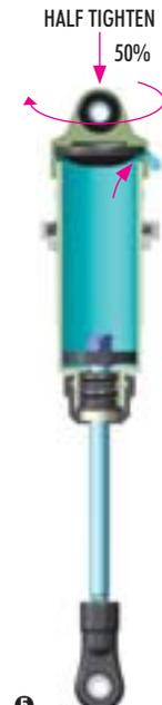
**5** Gently place the shock cap assembly onto the filled shock body. Excess oil will spill from the shock. Screw the shock cap onto the body by only a few turns.
