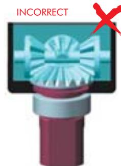
After assembly the differential should have a length of 32.6–32.7 mm measured from the ends of the installed ball-bearings. If differential is longer, retighten the 4 screws holding the spur gear.
