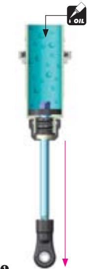
**1** Extend the shock shaft completely. Fill the shock body with the shock oil. For the FRONT shocks (short) use 600cSt oil. For the REAR shocks (long) use 350cSt oil.
