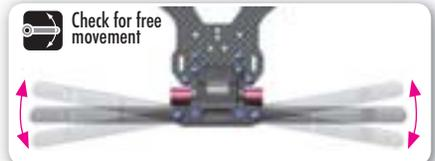
**!** Do not overtighten the self-locking nut. Overtightening may result in suspension binding.
