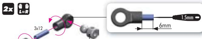
**TIP** Follow the TECH TIP on page 5 to install the pivot balls
