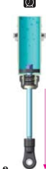
**3** Orient the filled shock vertically for several minutes with the shock shaft fully extended. The remaining air bubbles will release.
