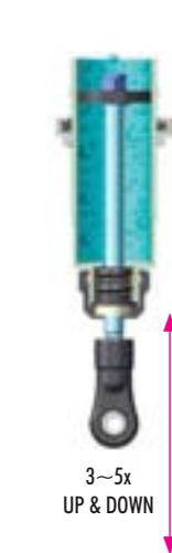
**2** Move the shock shaft up and down a few times to release the air bubbles trapped beneath the piston.
