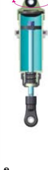
**7** Keep the shock shaft pushed in the shock body and tighten the shock cap completely. The rebound will be at approximately 0%.
