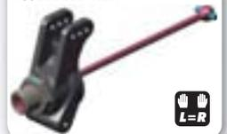
**TIP** Ensure that the rear upright moves freely. If it does not move freely, use sandpaper to thin both wheelbase adjustment shims.
