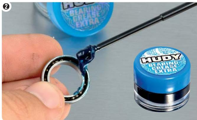
Use cleaner to get the dirt out of the bearing. After that, clean the bearing with a clean rag. Regrease the bearing with sufficient grease to fill the whole side.
