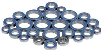
This is especially important with the bearings in the pinion gear assembly as they can carry extreme loads. We recommend using HUDY Bearing Grease after each hour of racing; this will help to significantly extend bearing life.
