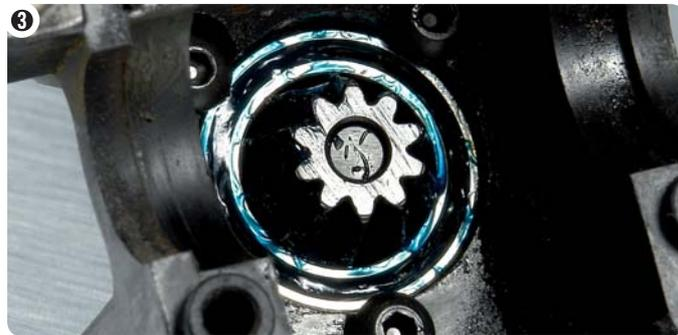
After the bearing is regreased and reinstalled, it is ready for use again.
