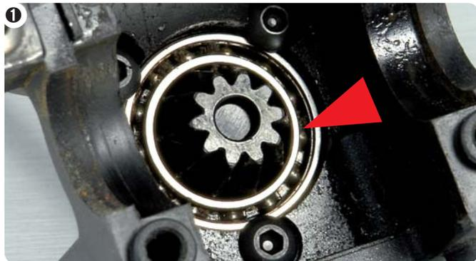
Bearing grease will disappear after some racing time. You must open the diff housing to access the bearing. Remove the bearing.
