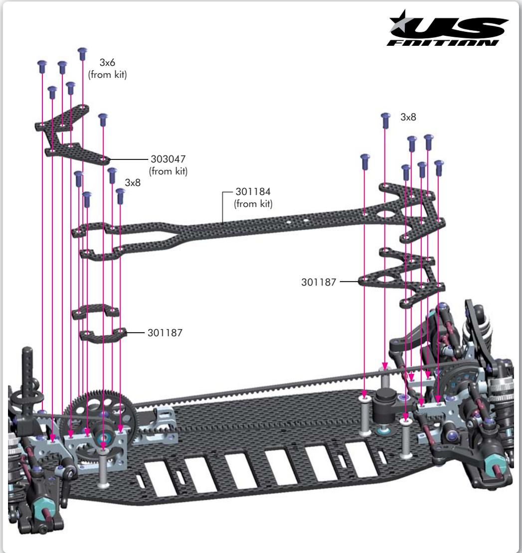
**NOTE!** The LiPo Conversion Set allows for the fitting of popular LiPo battery packs with a height of 24.5mm or less (the most popular and common configuration and sizing available on the market at the time of development). However, because of continuing development of LiPo batteries and no set of standardized regulations about battery sizes, XRAY cannot guarantee that all LiPo battery packs will fit in the US Edition cars using this conversion set.
