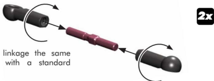
Make the linkage the same length as with a standard linkage.
