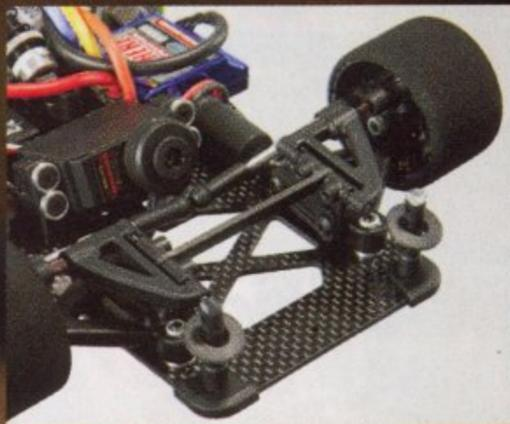
The front end has bumpers to protect the chassis from damage and fraying. The body mounts can be adjusted in fine increments to raise and lower the body. Two servo positions are
