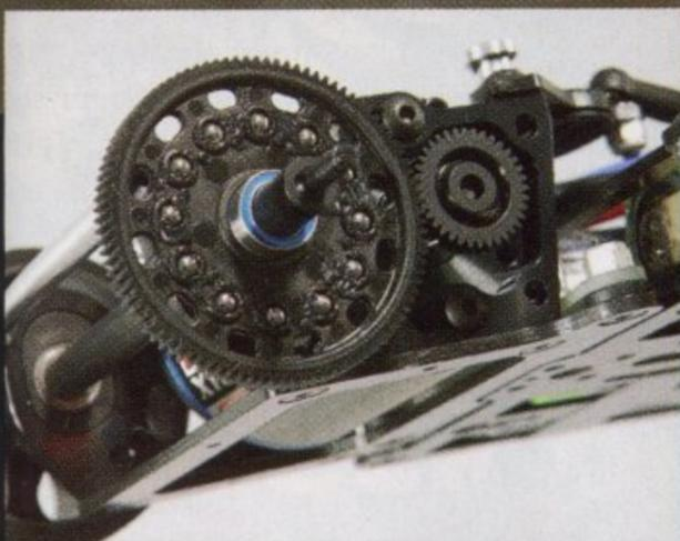
The graphite rear axle is precision-ground to reduce run-out. The diff plates mate with D-rings to prevent them from slipping. The black-anodized axle hubs have been machined to reduce their weight.
