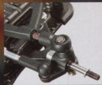
The X11's front suspension is molded in strong, yet flexible, composites to withstand hard impacts. Hudy Spring Steel pivot balls are used for smooth operation.
