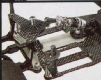
The included T-bar can be set up in two ways to suit either new drivers or advanced drivers. Setscrews let the driver adjust tweak.
