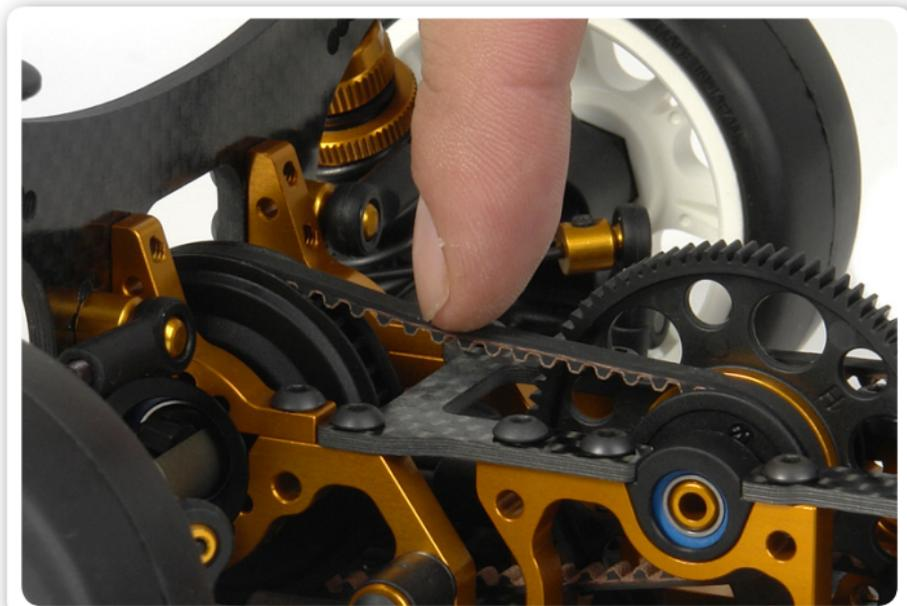
When the belts are mounted in the car for the first time, they will be tighter than the standard belts. Therefore we recommend you adjust the eccentric bushings so the belts are slightly looser, though it may happen that the belts still feel a bit tighter. Note that you can also use the #302077 1mm composite hubs for bulkheads to reduce the belt tension. The tension of the belts will not have a negative effect on the car's performance, and the belts will become softer after some run time.
