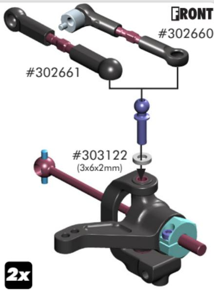
The new #302661 closed ball joints must be used with the new #302655 ball ends (optional ball ends are #302654 with 8mm thread and #302653 with 6mm thread). However, the new ball ends are designed to be used with standard #302660 open ball joints as well.
