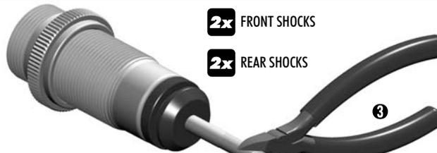
Grip the shock rod at top of exposed threads with side cutting pliers. Be careful not to damage the shock rod.
