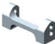
The optional 1-piece aluminum suspension holder is direct replacement for the standard rear holders of the front suspension. The 1-piece aluminum suspension holder will reinforce the chassis and will prevent chassis injury in serious crashes. The aluminum holder will make the front suspension a bit stiffer and will make the car slightly less steering responsive.
