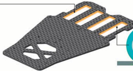
Do not file battery slots too much, or batteries may protrude below the chassis bottom.
