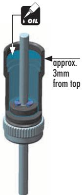
Extend the shock shaft completely to release the air trapped beneath the shock piston. Fill the shock shaft body with the shock oil but not fully approx. 3mm from the top of the shock body.
