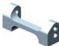
The 1-piece aluminum suspension holder is a direct replacement for the separate rear holders (#302046) of the front suspension. The 1-piece aluminum suspension holder reinforces the chassis and prevents chassis injury in serious crashes. The optional separate rear holders #302046 T3 ALU LOWER SUSPENSION HOLDERS can be used to gain more steering but will provide less stiffness.
