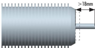
If shaft extends motor by more than 18mm, use the shim so the shaft does not touch the receiver box.
