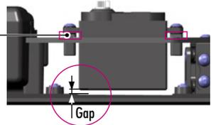
Use appropriate shims to ensure there is a gap between the servo and the chassis side guard.
