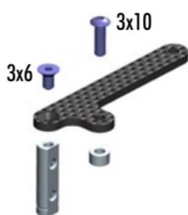
The new Center Servo Mount made from graphite allows the servo to be mounted to the chassis without touching it. The servo is mounted using three stands and without any other modifications. With this new servo mounting method, unwanted chassis tweak is eliminated while at the same time it provides more overall traction. The new servo mounting position improves the balance of the car as the servo is mounted more in the center of the chassis.
