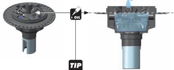
Fill differential up to the top of the diff pin. DO NOT fill the diff to the top of the housing.
