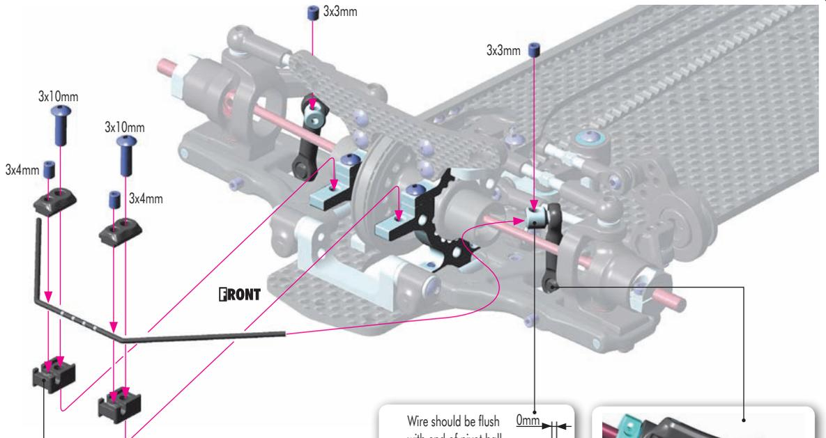
**IMPORTANT!** Only tighten enough to remove excessive free play; anti-roll bar must move freely.
