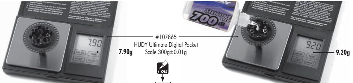
❶ Put the diff (without oil) on the scale and check the weight (approximately 7.90g)
