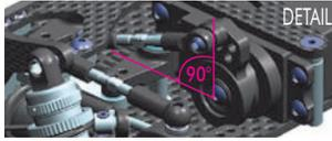
Attach servo arm to servo output shaft using screw from servo. Servo saver must be perpendicular to chassis when servo is in neutral.
