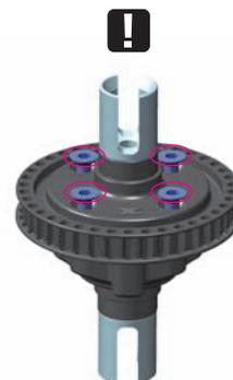
Tighten the screws equally but do NOT tighten them completely.
