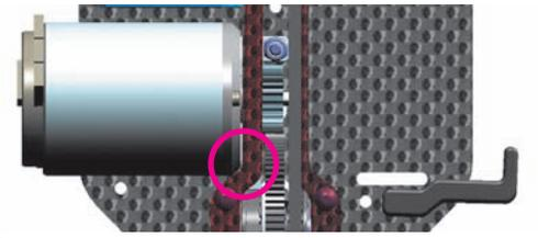
**TIP** For tightening and loosening the pinion set screw, use the indicated chassis hole.
