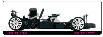
Ride height is the height of the chassis in relation to the surface it is sitting on, with the car ready to run. Ride height affects the car's traction since it alters the car's center of gravity and roll center. Because of changes in suspension geometry and ground clearance, there are negative consequences to altering ride height too much.
