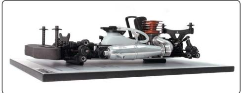
Place the droop gauge support blocks on the setup board, and then place the chassis on the support blocks.
