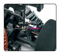
You may also adjust the rear anti-roll bar stiffness by using rear anti-roll bar wires of different thickness:
