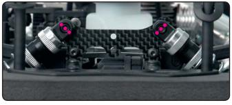
IMPORTANT: For each pair of front/rear shocks, the shock positions must be the same on left and right sides of the car.
