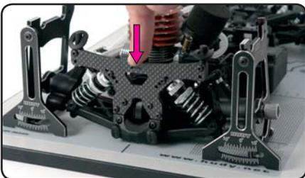
4. Push down and release the front and rear of the car so that the suspension settles.
