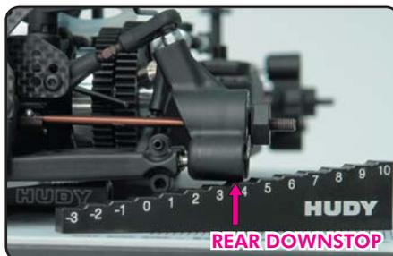
Downstops limit how far the suspension arms travel downward, which determines how far upward the chassis rises. This affects the car’s handling (due to effects on camber and roll-center) and the ability of the tires to “follow” the track. The effects may change with the type of track and/or amount of grip available.
