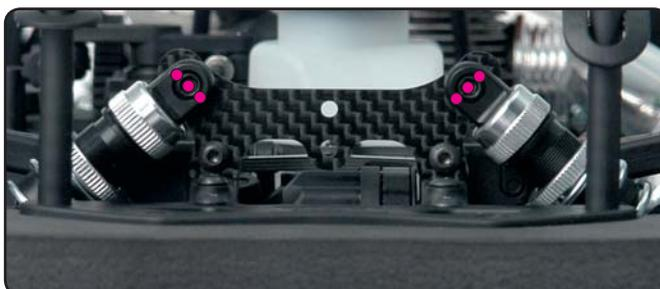
**IMPORTANT:** For each pair of front/rear shocks, the shock positions must be the same on left and right sides of the car.
