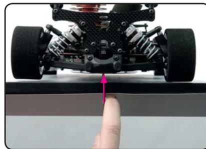
3. Adjust the preload on the FRONT springs until both rear wheels lift at the same time.
