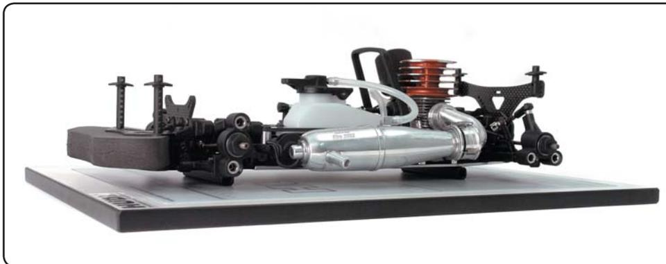
1. Place the droop gauge support blocks on the setup board, and then place the chassis on the support blocks. Make sure the chassis is solidly mounted on the support blocks so it does not move.
