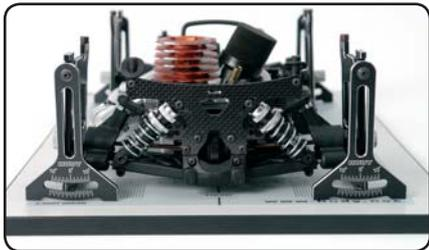
5. Read the camber setting from the camber gauge of each of the four set-up stands.
