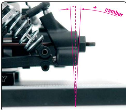
Camber is the angle of a wheel to the surface on which the car is resting (with wheels and shock absorbers mounted).
