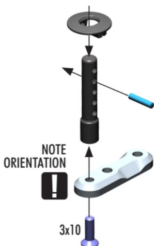
The Alu Bodymount Support is 4mm high, which is the same as the distance between holes in the body post. Therefore, lower the pin in the body post by 1 hole position.
