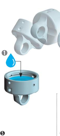
5 Fill the shock cap - fill the oil up to the o-ring.
