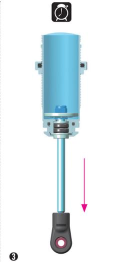
3 Orient the filled shock vertically for several minutes with the shock shaft fully extended. The remaining air bubbles will release.
