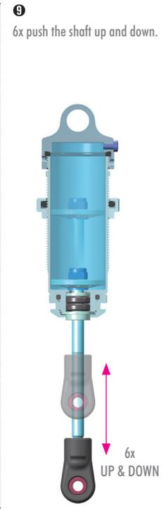
9 6x push the shaft up and down.
