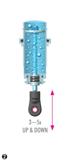
2 Move the shock shaft up and down a few times to release the air bubbles trapped beneath the piston.
