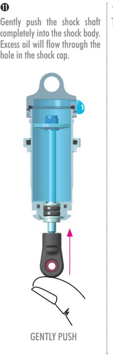
11 Gently push the shock shaft completely into the shock body. Excess oil will flow through the hole in the shock cap.
