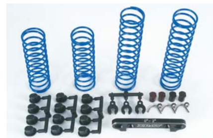
Xray supply these no-cost options to tune the chassis of the XB8
