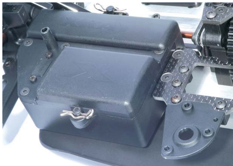
Two covers go over the receiver and the battery box should be close to watertight
