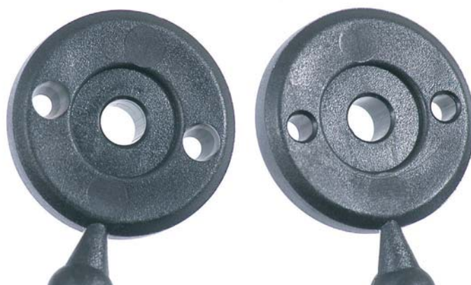
The shock piston on the left has a tapered hole, by altering its direction you can vary the bump and rebound characteristics
