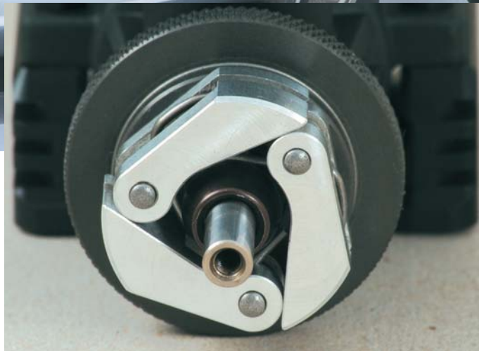
A three shoe alloy clutch does give amazing bite, Xray include two sets of springs to tune the bite point
