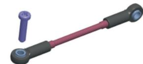
❸ Re-assemble the lower front drag link using the indicated shims and screws.
