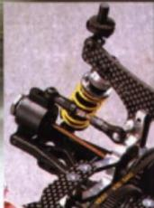
The short-arm suspension returns from the FK04 but is now crowned with an all new shock tower that adds a hole and moves the shocks out farther.
