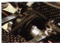
XRAY creativity at its finest. The FK05 comes standard with the new Multi-Diff. By sliding in a simple pin, you can go from full one-way, solid one-way, to locked spool.
