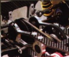
New, low CG bulkheads house larger pulleys that make the drivetrain extremely free.
