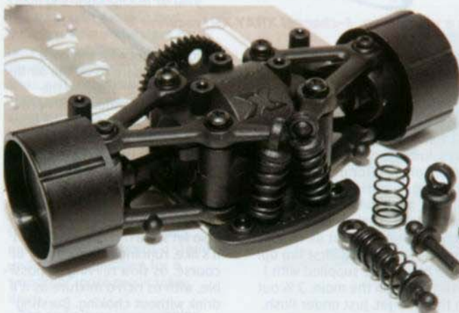
Simple shocks have two positions for balancing the handling
