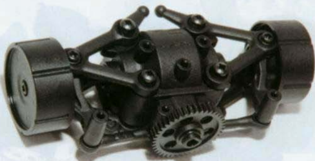
Fully assembled rear end, note two sets of wheel attachment slots to alter track width
