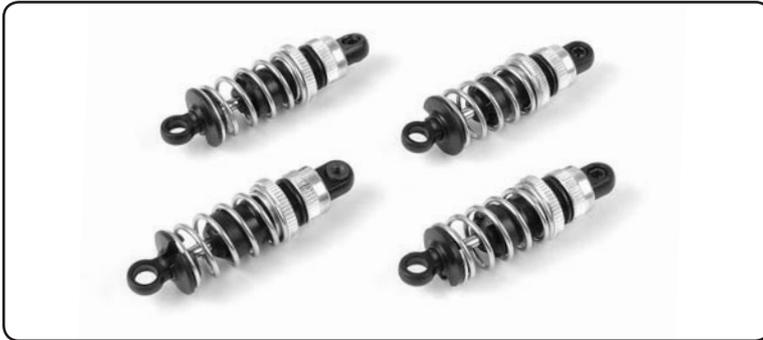
The most important factor for a tweak-free car is to have left with right shocks set up perfectly equal with springs. Both pairs of shocks must have:
