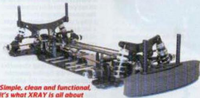
Spacers under inboard pivots set inboard rear toe. The hole in diff allows slip adjustment in situ
