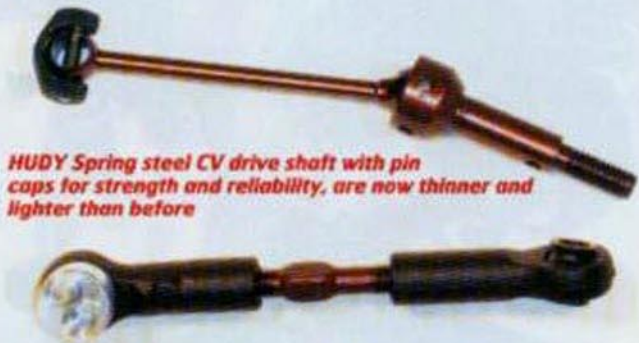
The cool new eccentric camber link mounts for quick roll centre adjustments - it really works!
