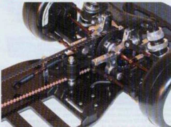
Turnbuckles throughout for accurate set up, and Hudy Spring steel components build confidence
