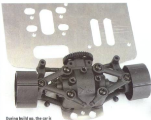
During build up, the car is constructed in modules - here you can see the rear end attached to the chassis
