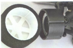
The wheels slide into place onto these grooved hubs
