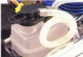
Above: the 30cc tank contains enough fuel to keep the engine running for 6 minutes or more. It also has a built-in stone filter to ensure that the fuel that reaches the carb is clean.
