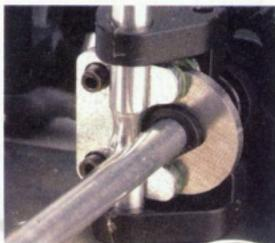
Left: the brake rotor is laser-cut and hand ground to tight tolerances, and the steel calipers have Ferodo brake pads for smooth, consistent braking.
