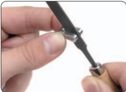
To ensure the proper fit of these spring in the clutch shoes, you will need to slightly hand-modify the groove in each shoe. Use a thin file to enlarge the width of the groove. **DO NOT** use a knife. Make sure to use proper eye and hand protection.
