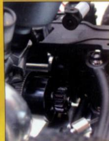
and although there isn't any supplied grease—nor does it specify to use any lubricant on the pinion and crown—I did apply a smear of light automotive grease to them.
