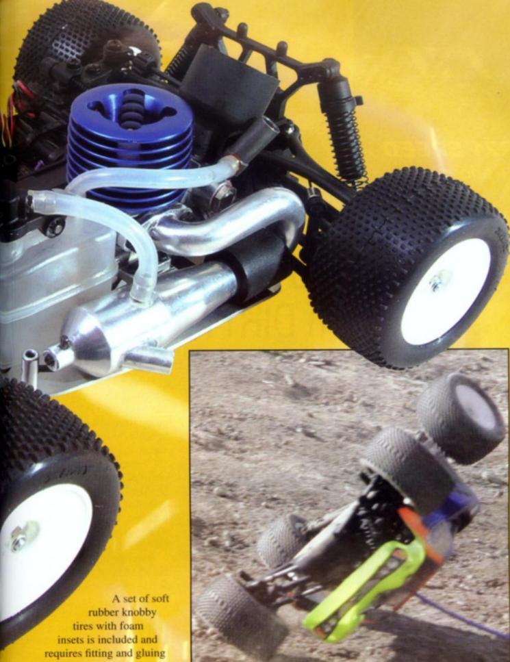
A set of soft rubber knobby tires with foam insets is included and requires fitting and gluing onto the rims.
