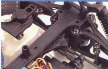
A one-bellcrank steering system points the wheels where you want them to go. Ball bearings ensure smooth performance. The heavy-duty servo-saver protects the steering servo.
