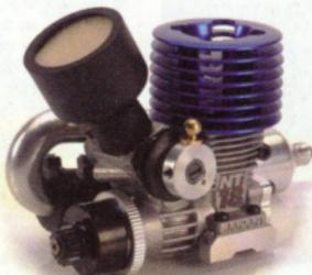
The XRAY 0.8cc engine is powerful and reliable. It has a dual-needle slide carb and a big, machined-aluminum cooling head just like larger engines. The engine does not have a pull-start mechanism, so you'll need a starter box.
