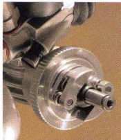
An aluminum two-shoe clutch is included to engage the steel 16t clutchbell. A starter box is required to spin the small aluminum flywheel.
