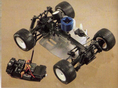
Team Xray's Micro Electronic Pack includes the two micro servos, a receiver battery pack and the on/off switch. Those and the receiver all mount nicely to the radio tray that is removed as a single unit for ease of maintenance.
