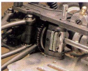
The steel spur gear is mounted directly in front of the rear diff. A single steel disc is used for braking. The Ferodo pads showed no signs of fade after many tanks of fuel. The center driveshaft is made from aluminum and distributes power from the .08cc engine evenly to the front and rear. You can also see the engine's low speed needle—yes, it has a dual-needle carb.
