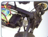
The smooth bearing filled steering system has plenty of power from the 6V hump pack
