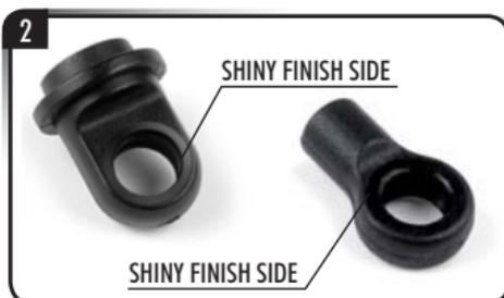
The lower composite ball joints and upper shock eyelets have two sides. One side has a shiny finish on the area around the pivot ball hole, while the other side has a regular finish.
