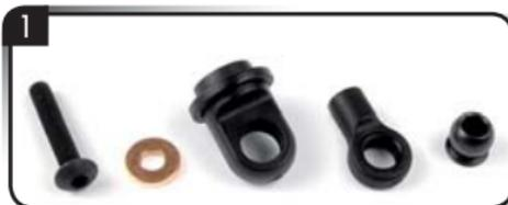
To install 5.8mm balls into composite ball joints follow this handy tip. From the Last Aid bag, get a M3x16mm SH screw, a 3x7.5x1.13 yellow shim. Also get the #303241 pivot balls and the #308316 ball joints and upper shock eyelets.
