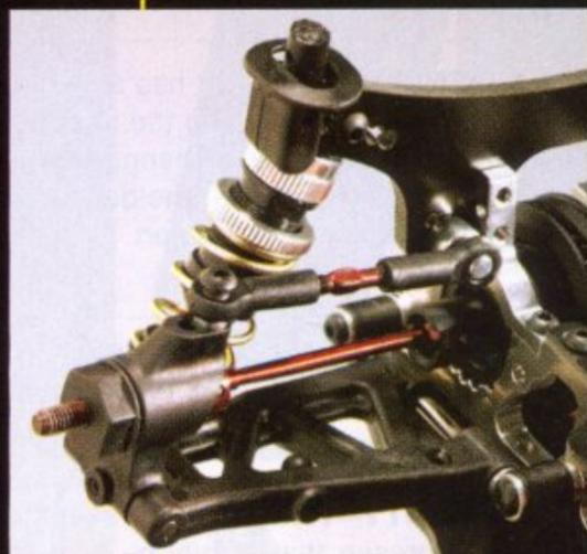
The rear hub carriers and arms are made extra sturdy to withstand impacts. Here you can see that the hinge pin block can be easily accessed for added tuning. Wheelbase may also be changed with the included spacers.
