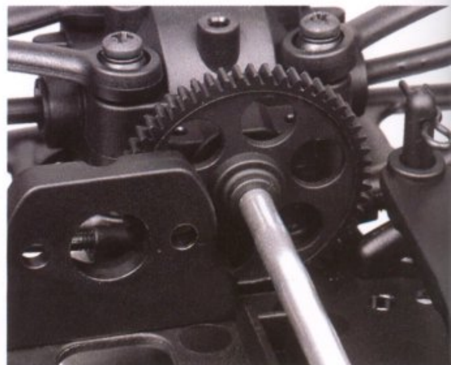
54 tooth spur gear mounts directly onto the solid aluminium drive shaft to give the 4WD action
