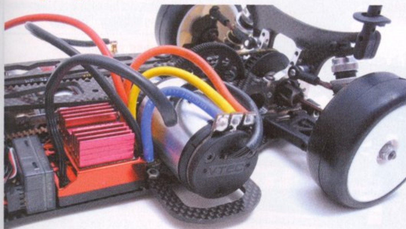
See the Multi-Flex slots which the upper plate and link posts control
