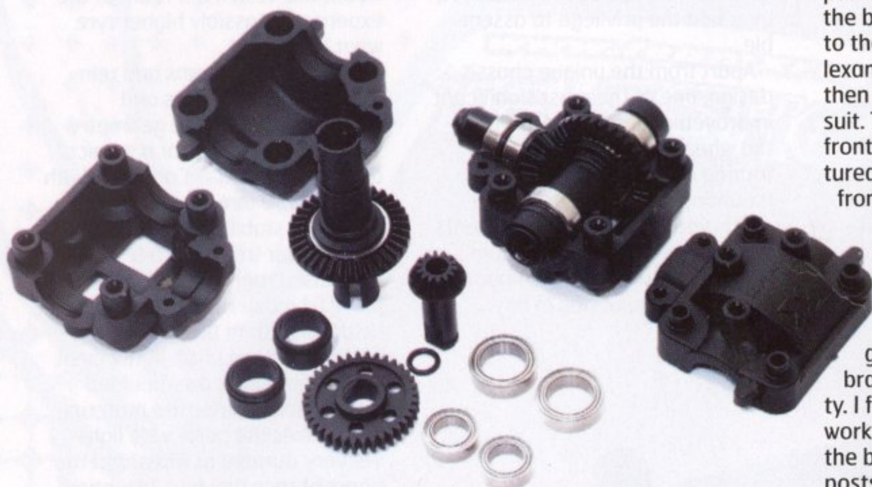
Pre-built ball differentials slot straight into diff cases
