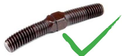
Please note that the hardness of the front upper turnbuckles has been modified for the XB8EC kit; the new turnbuckles are purposely softer. In the event of a serious crash, the softer material will allow the turnbuckle to bend slightly instead of breaking; this will help allow you to finish the race.
